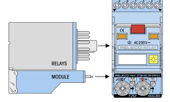
**The system sockets** C12B0 or C-155 serve as a basis for the secure reception of the electronic modules. The sockets have a 4-pole module slot in which the CT modules lock firmly and vibration proof also without the output relay. Contact is made with reliable twin knife contacts.
