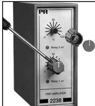
Picture 2: Removal of knobs.
